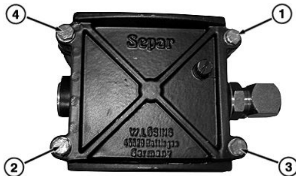
Lid Cap Screw Tightening Sequence
