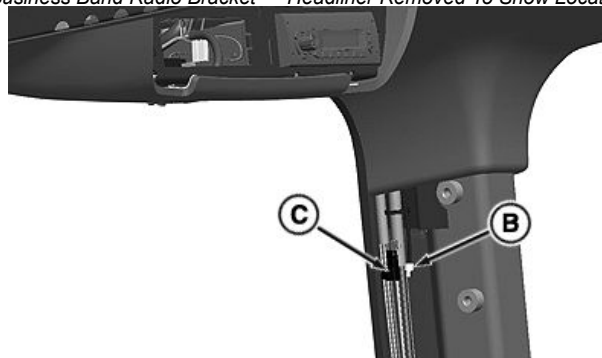
Antenna Coaxial Cable And Business Band Radio Power/Ground plug Coiled Behind Right Rear Corner Post Cover
