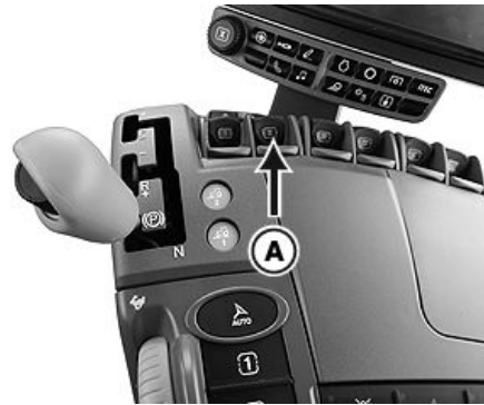
SCV Control Lever Retract and Retract Detent
