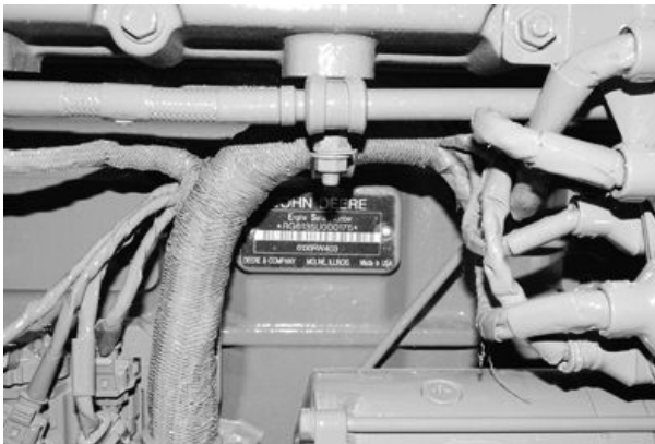
13.5 L Engine Serial Number Plate Location
