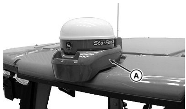
StarFire™ Receiver Mounted on StarFire™ Receiver Bracket
