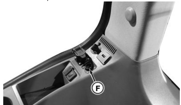
ISO 11783 Connector on Right-Hand Console
