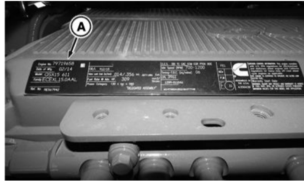
15 L Engine Serial Number Plate Location
