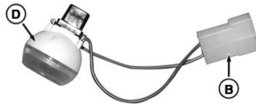
Remove Bulb From Retaining Ring
