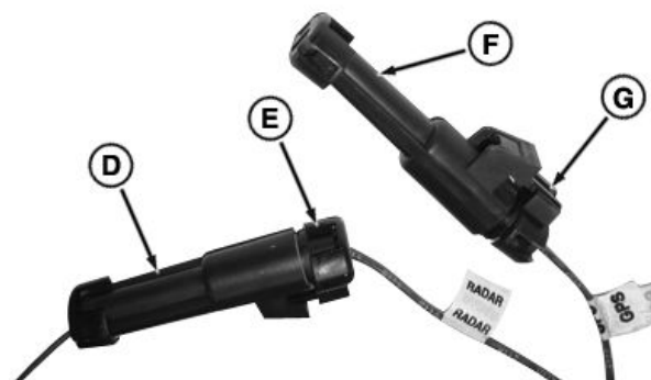
Connectors For Radar and GPS
