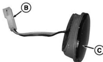
Remove Bulb From Retaining Ring
