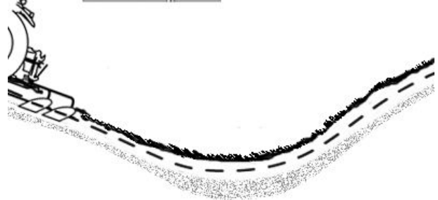
Higher Response Causes Better Depth Control In Rolling Terrain
